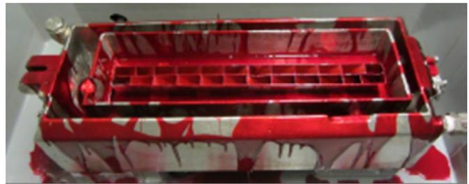
**Fig. 1** Part of an encapsulation system: considerable criticality due to the assembly of the parts into a single body, which cannot be disassembled for the treatment.
