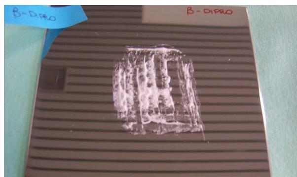
**Fig. 2** Dirty coupon with Diprostene - Fine-tuning of a machine part cleaning process at the R&D department of Fedegari
